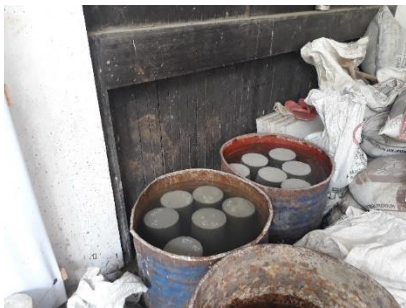
Gambar 33. Rawatan keras metode water submerged
